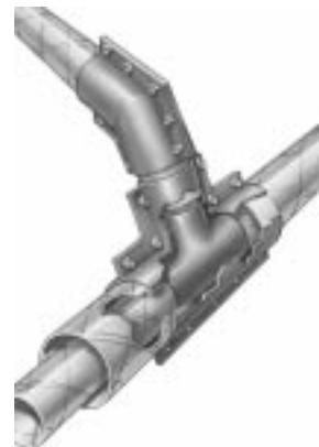
Figure 4 - Example of FRP Double-Walled Piping
